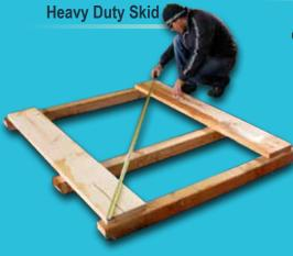
A counter sunk carriage bolt at four corners secures a Heavy Duty deck to each skid...
